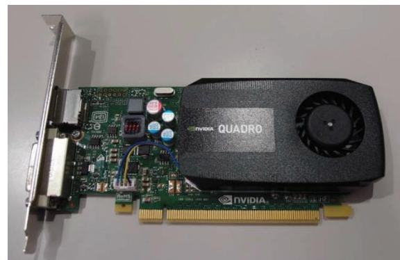
Picture 1. PCI Express x16 Graphics Card (NVIDIA Quadro K420)
